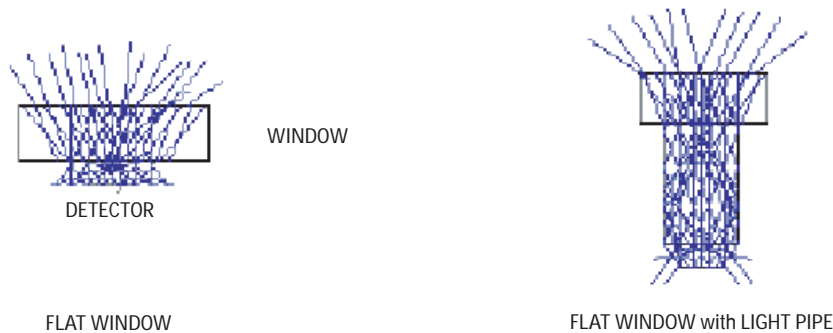
Figure 12. Recommended window design.
