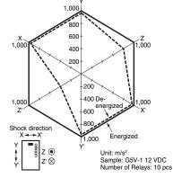
Test conditions: Shock is applied in ±X, ±Y, and ±Z directions three times each with and without energizing the Relays to check the number of contact malfunctions.
