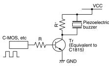
$^{*}$  Resistor to do charging and discharging to a piezoelectric element (Value of about 1k $\Omega$  is good efficiency).
