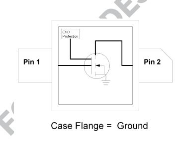
Note 1: Gate voltage must be applied to  $V_{GS}$  lead concurrently or after application of drain voltage to prevent potentially destructive oscillations. Bias voltages should never be applied to the transistor unless it is properly terminated on both input and output.
