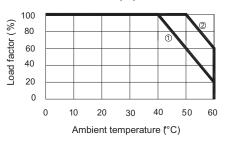
① Convection @ Forced air (0.5m³/min) (18 CFM)
