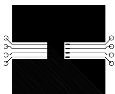
a) 50^\circ\text{C/W} when mounted on a 1\text{ in}^2 pad of 2 oz. copper.
