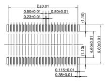
Recommended metal mask pattern Metal mask thickness: When 120 µm (Opening area ratio: 69%)
