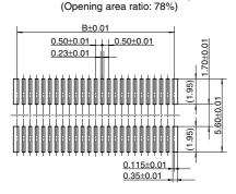
\* See the dimension table on page 5 for more information on the B dimension of the socket and header.
