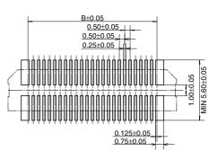
Recommended metal mask pattern Metal mask thickness: When 150 μm (Opening area ratio: 62%)
