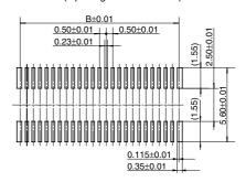
Recommended metal mask pattern Metal mask thickness: When 120  $\mu$ m
