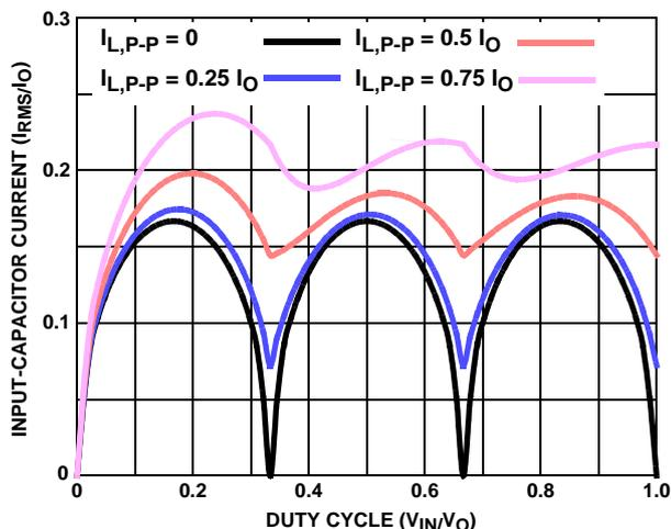
**FIGURE 24. NORMALIZED INPUT-CAPACITOR RMS CURRENT FOR 3-PHASE CONVERTER**
