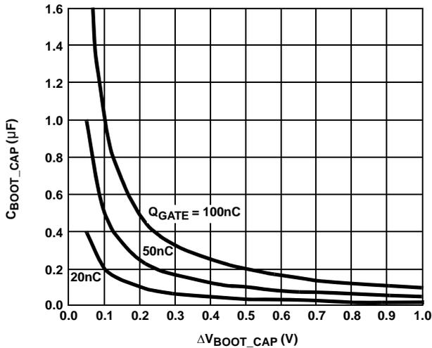
**FIGURE 10. BOOTSTRAP CAPACITANCE vs BOOT RIPPLE VOLTAGE**
