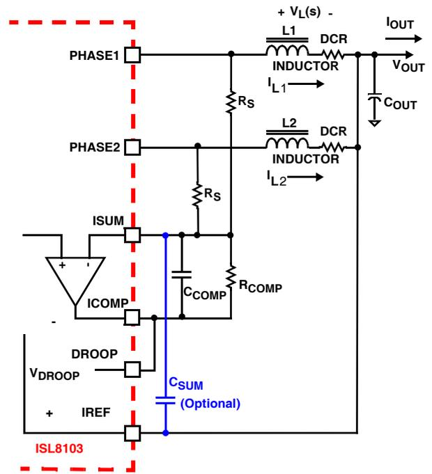
**FIGURE 7. DCR SENSING CONFIGURATION**
