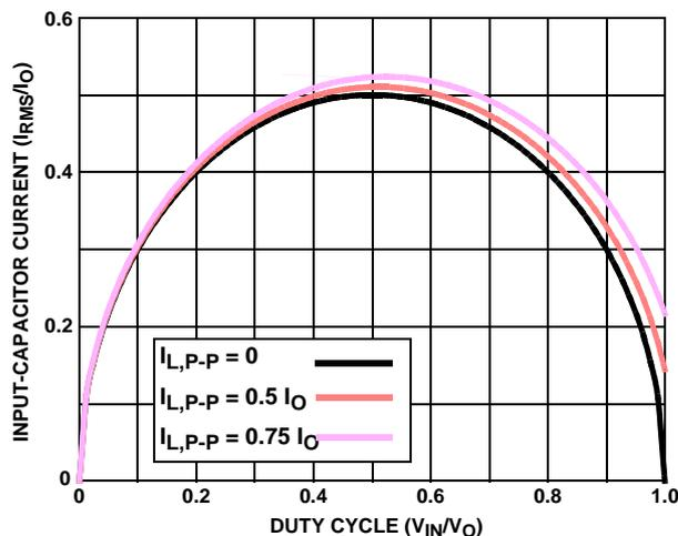
**FIGURE 26. NORMALIZED INPUT-CAPACITOR RMS CURRENT FOR SINGLE-PHASE CONVERTER**
