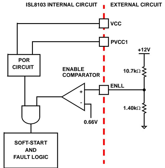
**FIGURE 11. POWER SEQUENCING USING THRESHOLD-SENSITIVE ENABLE (ENLL) FUNCTION**
