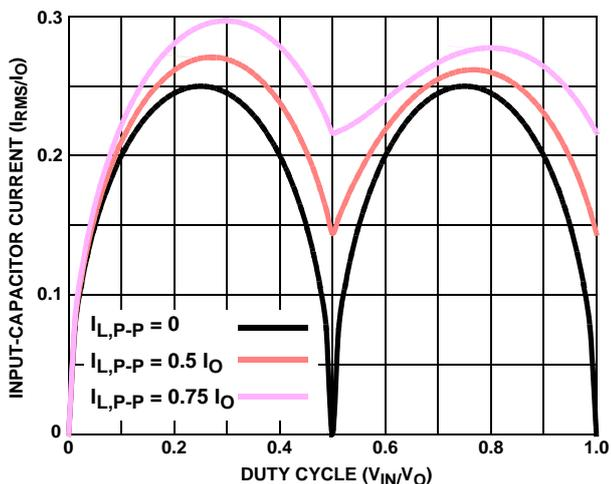
**FIGURE 25. NORMALIZED INPUT-CAPACITOR RMS CURRENT FOR 2-PHASE CONVERTER**
