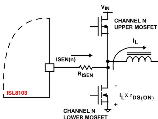
FIGURE 17. ISL8103 INTERNAL AND EXTERNAL CURRENT-SENSING CIRCUITRY
