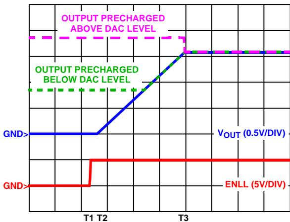
**FIGURE 12. SOFT-START WAVEFORMS FOR ISL8103-BASED MULTIPHASE CONVERTER**
