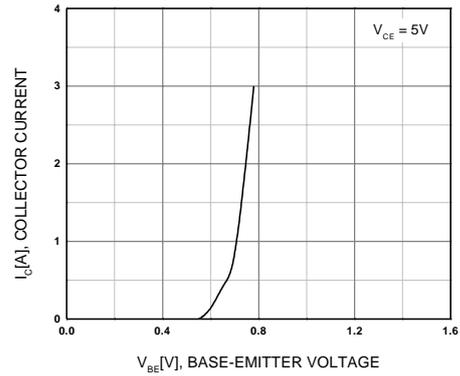
**Figure 4. Base-Emitter Voltage**
