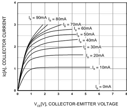
**Figure 1. Static Characteristic**
