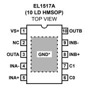
THERMAL PAD MUST BE CONNECTED TO GROUND. PAD IS CONNECTED INTERNALLY TO  $V_S\mbox{-}$  AND THUS EL1517A CAN ONLY BE USED IN SINGLE SUPPLY APPLICATIONS.
