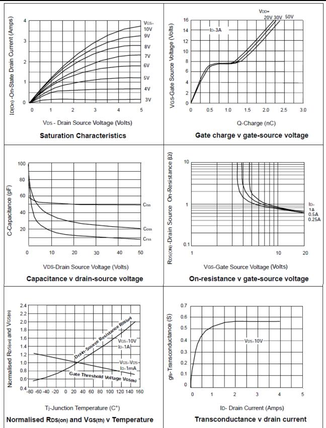
Datasheet of ZVN2106GTA - MOSFET N-CH 60V 710MA SOT223
