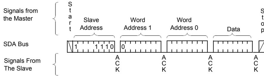
**Figure 9. Writing 30 bytes to a 128-byte memory page starting at address 105.**
