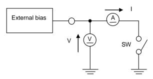
External bias voltage shall be measured when SW left open.
