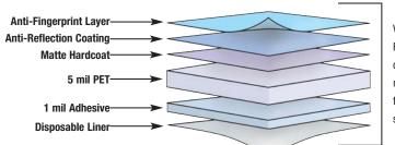
Vikuiti Removable Anti-Reflection Film's unique multilayered construction reduces glare, makes it easier to wipe off fingerprints and helps shield screens from scratches.
