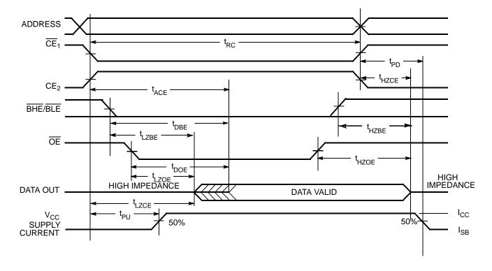
19. The device is continuously selected.  $\overline{OE}$ ,  $\overline{CE}_1 = V_{IL}$ ,  $\overline{BHE}$  and/or  $\overline{BLE} = V_{IL}$ , and  $\overline{CE}_2 = V_{IH}$ .
