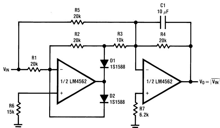
**Figure 122. AC/DC Converter**
