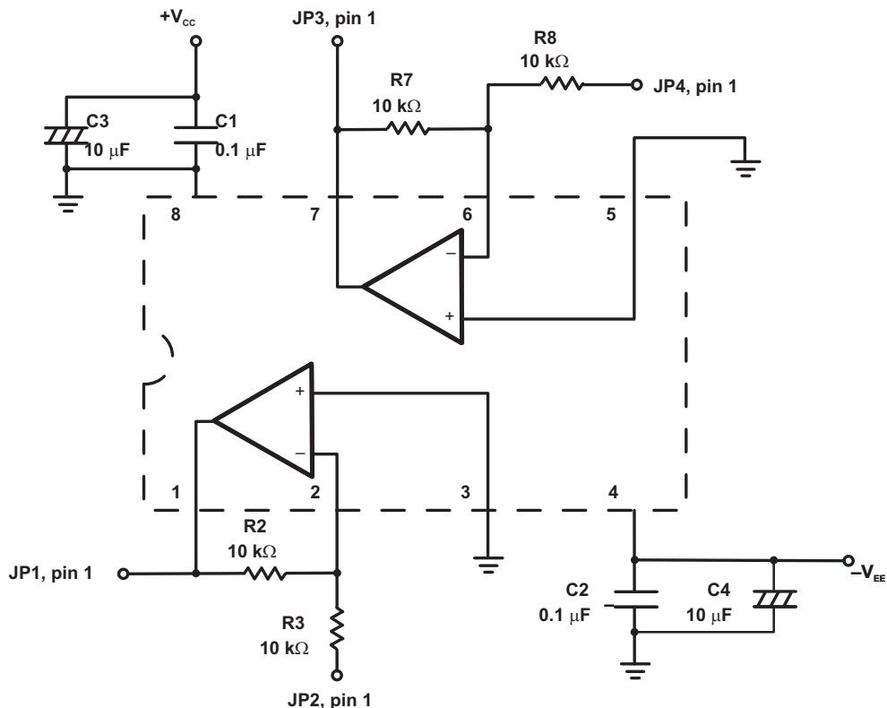
Figure 113. Inverting Amplifiers
