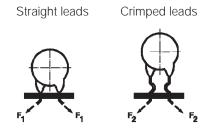
Maximum pull force during insertion and lead cut
