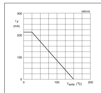
Device mounted on an FR4 printed-circuit board.
