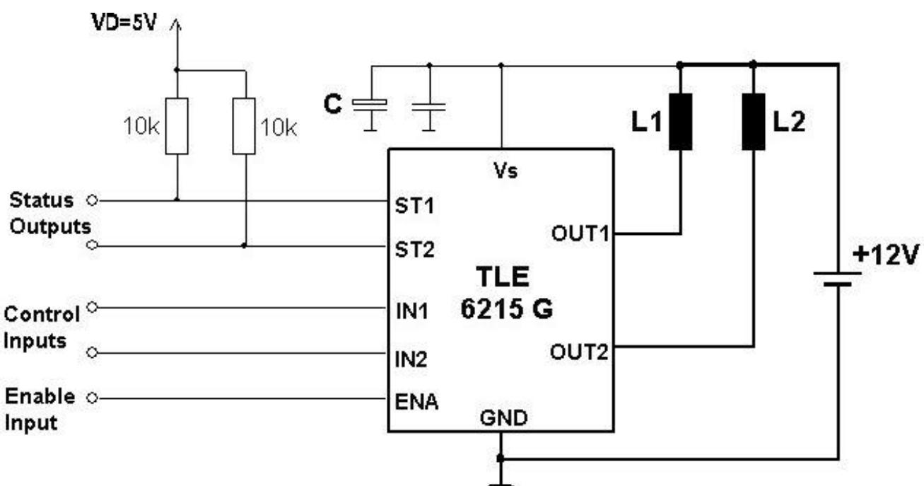
The blocking capacitor C is recommended to avoid critical negative voltage spikes on  $V_s$  in case of battery interruption during OFF-commutation.
