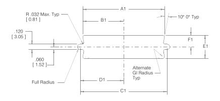
Strain Relief (Order Separately or with Connector) Material: Stainless Steel
