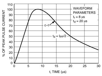
12.0 3 PULSE WAVEFORM IPP, PEAK PULSE CURRENT 8 x 20 μs per Figure 1 10.0 8.0 6.0 4.0 2.0 0.0 30 35 40 45 25 50 V<sub>C</sub>, CLAMPING VOLTAGE (V)
