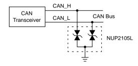
Figure 7. High–Speed and Fault Tolerant CAN TVS
