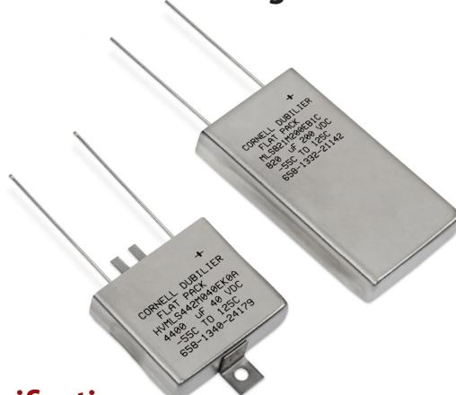
Encased in rugged stainless steel, the MLS is perfect for high reliability military systems and applications operating above 85 °C. For our highest performing 125 °C Flatpacks, choose type HVMILS available in a special stainless steel case for high vibration applications up to 50g. Specify type HRMLS for high reliability Flatpacks which are subjected to MIL level burn-in processes to ensure established reliability.
