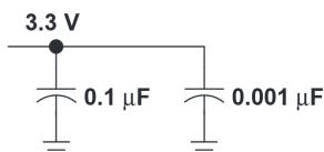
Figure 16. Recommended LVDS Bypass Capacitor Layout
