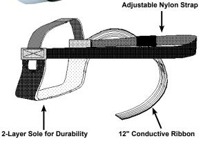
TG1M Toe Grounders are designed for use on standard shoes, including high heeled shoes. This quality Toe Grounder features a durable two-layer sole and an 12 inch multi-strand conductive ribbon. This item is UL listed and lot numbered. To be worn on both feet, but TG1M is sold one each.
