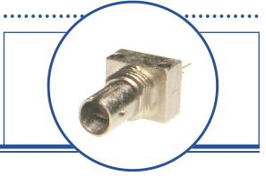
The OPF322 family fiber optic transmitters are high performance devices packaged for data communication links. This transmitter is an 850nm GaAlAs LED and is specifically designed to efficiently launch optical power into fibers ranging in size from 50/125µm up to 200/300µm diameter fiber. Multiple power ranges with upper and lower limits are offered which allows the designer to select a device best suited for the application.
