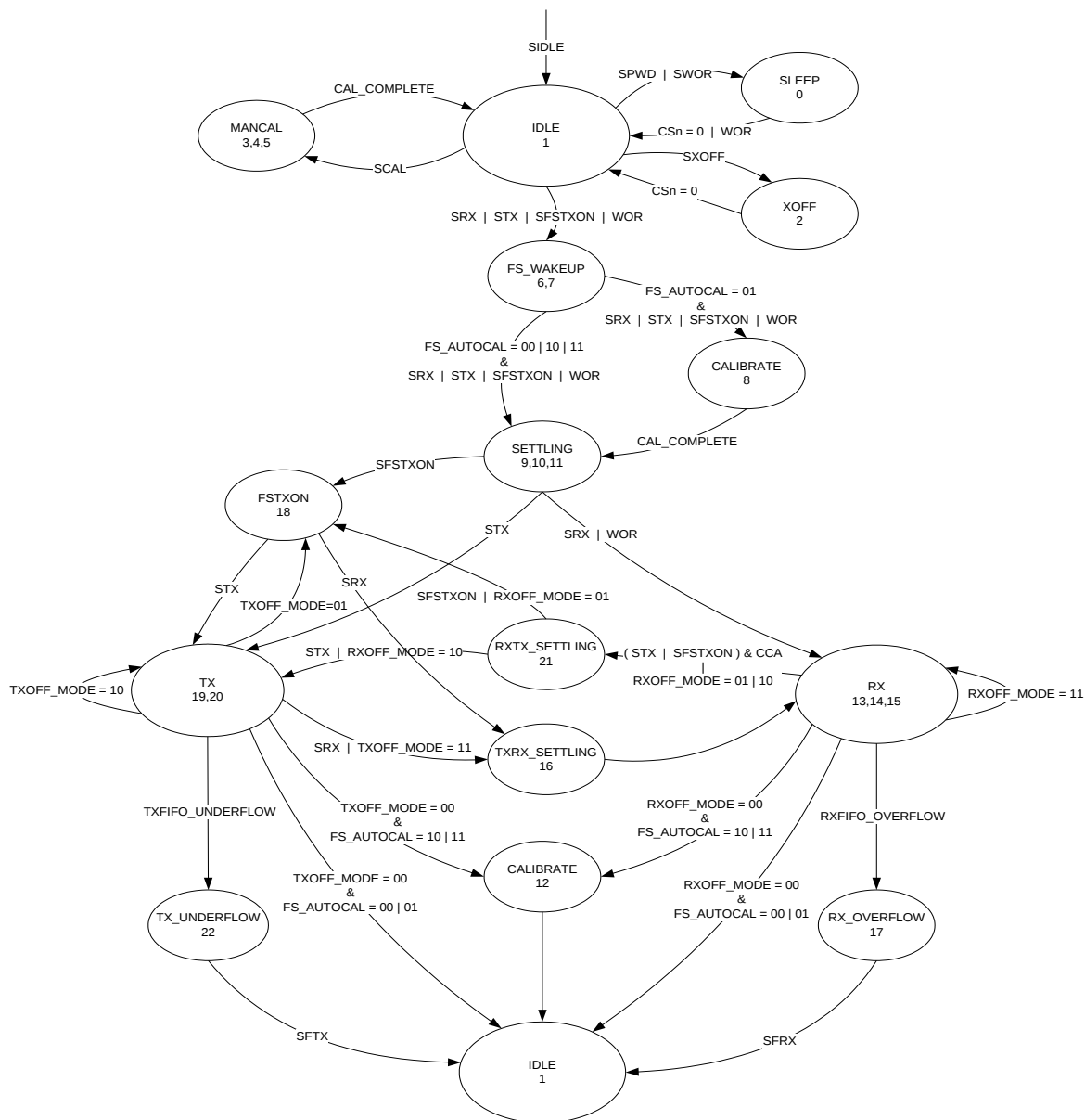
Figure 25: Complete Radio Control State Diagram
