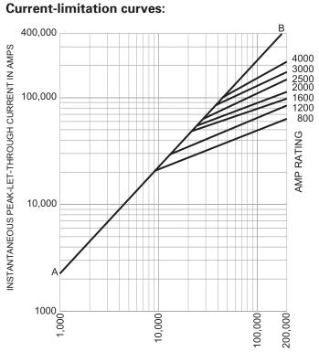
RMS SYMMETRICAL CURRENT IN AMPS A-B = ASYMMETRICAL AVAILABLE PEAK (2.3 X SYM RMS AMPS)
