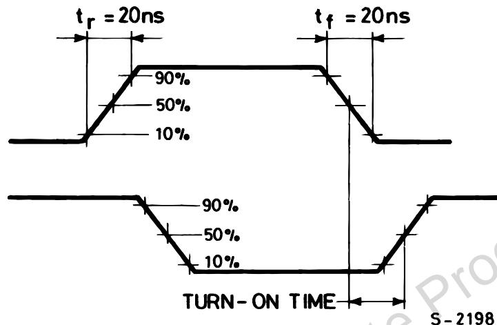
**WAVEFORM : PROPAGATION DELAY TIMES (f=1MHz; 50% duty cycle)**
