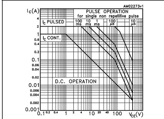
Figure 3. Derating curve
