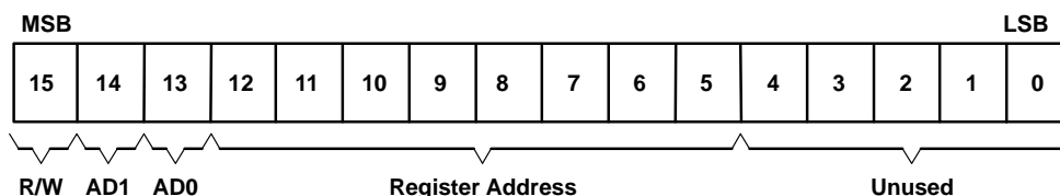
Figure 5. Bit Assignment and Definition for Slot 0 Word
