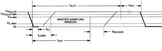
$60 \ \mu s \le t_{SLOT} < 120 \ \mu s$   $1 \ \mu s \le t_{LOWR} < 15 \ \mu s$   $0 \le t_{RELEASE} < 45 \ \mu s$   $1 \ \mu s \le t_{REC} < \infty$   $t_{RDV} = 15 \ \mu s$   $t_{SU} < 1 \ \mu s$
