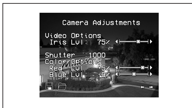
Figure 2. CVBSOUT with the Second OSD Display in Demo Mode (NTSC)
