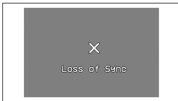
Figure 3. CVBSOUT in Demo Mode During LOS (NTSC)
