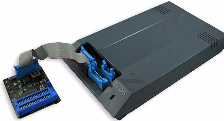
Figure 3. OTP Programming Adapter (Included with the Crimzon ICE)
