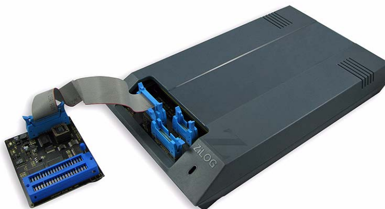
Figure 5. OTP Programming Adapter (Included with Crimzon ICE)
