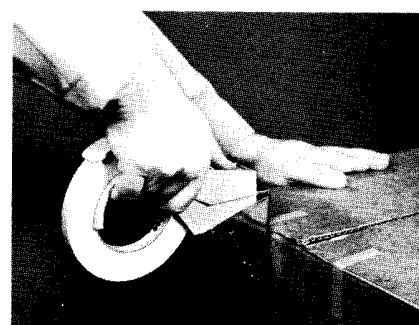
Figure 5 — With brake tension on the tape roll, push the H-131 straight downward to cut the tape and buff it against the box to complete the application.
