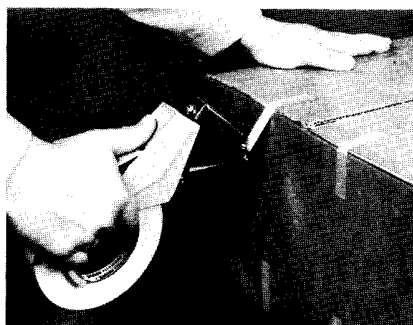
Figure 4 — Pull the H-131 over the box edge to dispense about 2 inches [50 mm] of tape as shown. Apply tension on the brake, tilt the H-131 upward, and tuck the tape to the side of the box with the top buff pad to form a tight seal.
