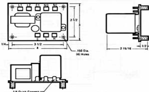
This is a fixed-sensitivity, forward mode control. The control relay is energized when liquid rises to contact the "H" probe. The control relay is pulled in and remains energized until liquid drops below the "L" probe.
