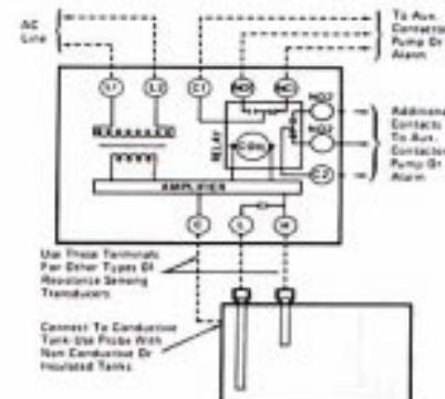
This is a fixed-sensitivity, forward mode control. The control relay is energized when liquid rises to contact the "H" probe. The control relay is pulled in and remains energized until liquid drops below the "L" probe.
