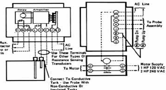
Model LCT is a forward mode control. The control relay is energized when liquid rises to contact the "H" probe. The time delay on operate is 3 seconds nominal and 0.5 seconds on release. Other values between 0.5 and 10 seconds are available on request. The control relay is pulled in and remains energized until liquid drops below the "L" probe. Sensitivity is adjustable.
