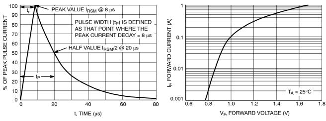
Figure 3.  $8 \times 20~\mu s$  Pulse Waveform
