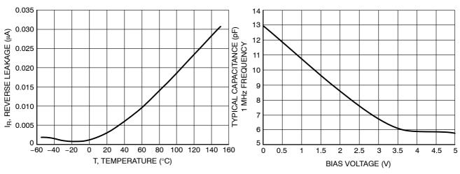
Figure 1. Reverse Leakage Current versus Temperature
