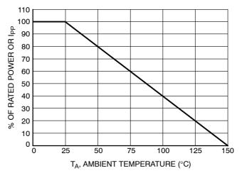
Figure 5. Power Derating Curve
