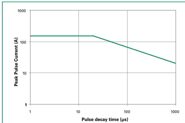
Figure 1: Non-repetitive Peak Pulse Current vs. Pulse Time
