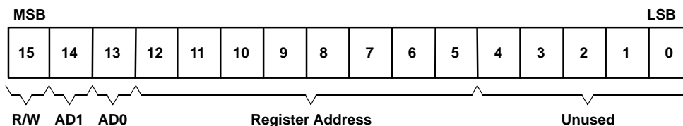
Figure 5. Bit Assignment and Definition for Slot-0 Word
