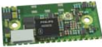
Picture 1: CB-OEMSPA331x-06 OEM Serial Port Adapter long range with external antenna and a JST 6-pol connector
