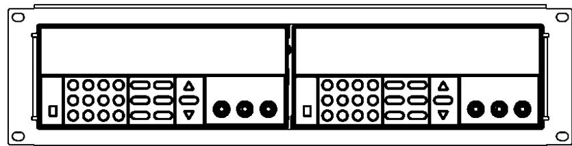
To rack mount two instruments side -by-side, order rack mount kit IT-E151, you
