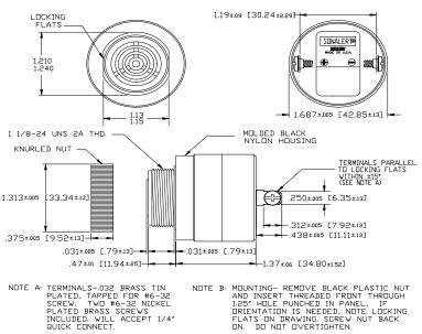
NOTE B: MOUNTING- REMOVE BLACK PLASTIC NUT AND INSERT THREADED FRONT THROUGH 1.25' HOLE PUNCHED IN PANEL, IF DRIENTATION IS NEEDED, NOTE LOCKING FLATS ON DRAWING. SCREW NUT BACK ON. DO NOT OVERTIGHTEN.
