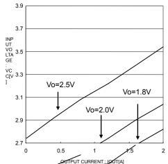
Fig.33 minimum input voltage in each output voltage
