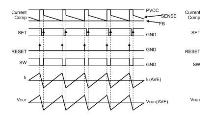
Fig.19 PWM switching timing chart
