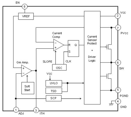
Fig.3 Block Diagram
