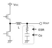
Fig.27 Output capacitor
