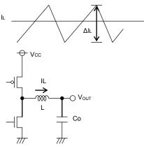
Fig.26 Output ripple current
