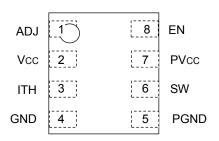
Fig.2 Pin Configuration
