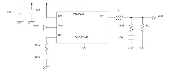
Fig.1 Typical Application Circuit
