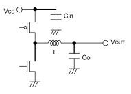
Fig.28 Input capacitor
