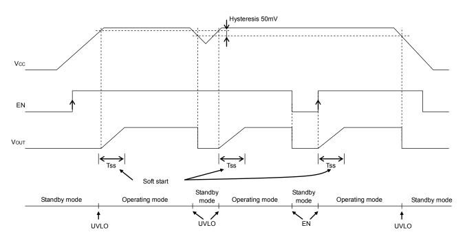
Fig.20 Soft start, Shutdown, UVLO timing chart
