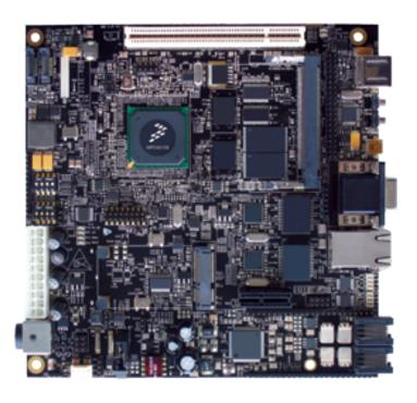
A board support package (BSP) is pre-installed on the MPC8315E-RDB. This BSP includes a bootloader (u-boot)—a generic Power Architecture technology system based on the Linux® kernel. The u-boot and Linux kernel reside in the on-board flash memory.
