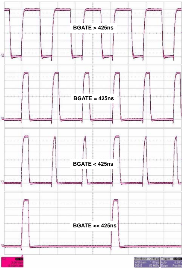
FIGURE 4. BGATE PULSE STRETCHING
