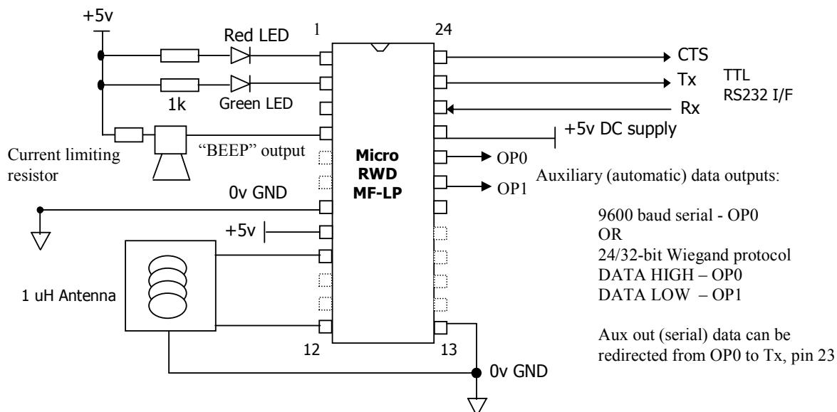
With the ultra-low-power current consumption and the additional auxiliary data output features, this one of the most compact and flexible reader systems available.
