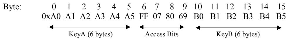
The default access bits (0xFF 07 80 69) define that KeyA must be used for all operations and KeyA can never be read, so in the previous example bytes 0 – 5 (keyA) would always read as zeros.
