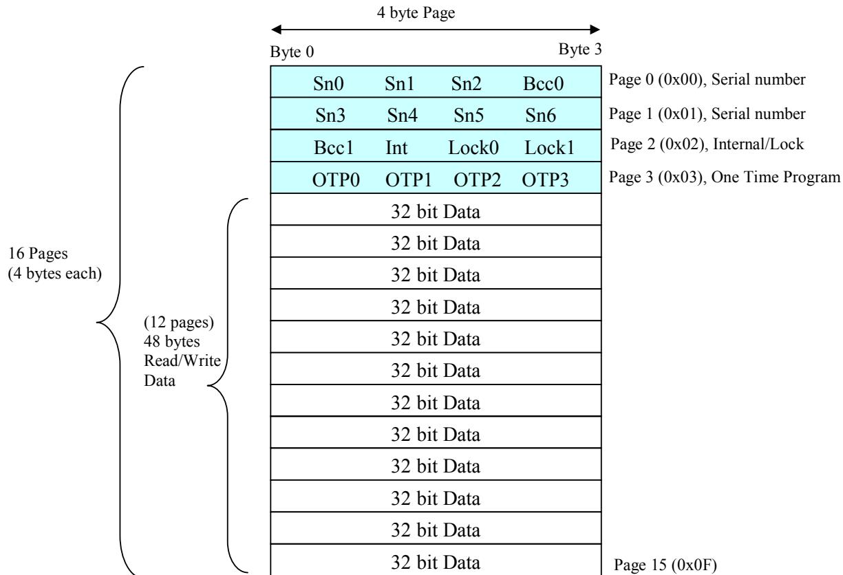
**Note:** Ultralight card has 7 byte serial number (+ 2 check bytes)
