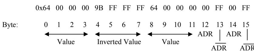
Note that the ADR and inverted ADR block address is part of the required format for the Value Data Structure BUT it is not changed by the Inc, Dec or Transfer commands and exists to allow optional storage of block numbers. For general use, the 0x00 address and 0xFF inverted address can be used to satisfy the structure format. The Inc, Dec and Transfer commands first check the structure format before beginning the operations and the commands fail if the format is not correct.
