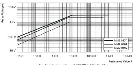
Pulse load rating in accordance with IEC 60115-1, 4.27; 1.2  $\mu$ s/50  $\mu$ s; 5 pulses at 12 s intervals; for permissible resistance change ± (0.5 % R + 0.05  $\Omega$ )
