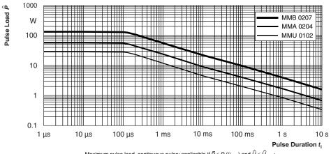
Maximum pulse load, continuous pulse; applicable if  $\bar{P} \leq P(\vartheta_{amb})$  and  $\hat{U} \leq \hat{U}_{max}$ ; for permissible resistance change ± (0.5 % R + 0.01  $\Omega$ )
