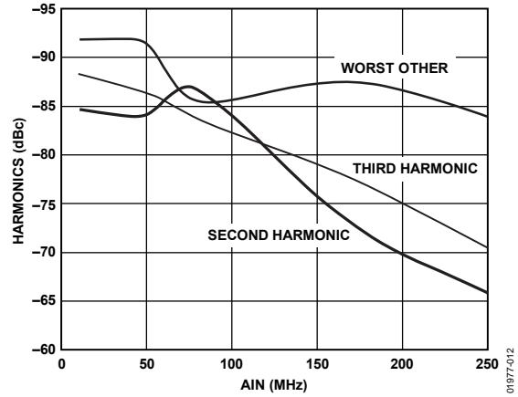
Figure 7. Harmonics (Second, Third, Worst Other) vs. AIN Frequency, AIN @ -0.5 dBFS, f_s = 105 MSPS, SFDR Mode Enabled
