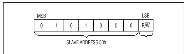
Figure 1. DS3503 Slave Address Byte
