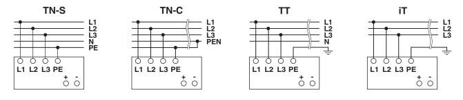
The connection for 3x 400 V AC ... 500 V AC is achieved using the L1, L2, L3 and PE screw connections. The device can be connected to 3-phase systems with nominal voltages 3x 400 V AC ... 500 V AC are connected. In the event of a phase failure, unrestricted operation is possible with nominal capacity. An operation in DC networks is also possible without any limitations.
